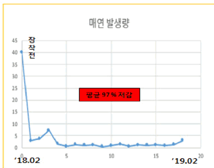
Fig. 4 reduction of soot with DPF regenerated by plasma burner
